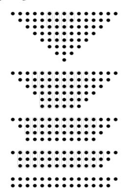
Fig. 7. Reduction circuitry of an 8-bit Dadda multiplier.
