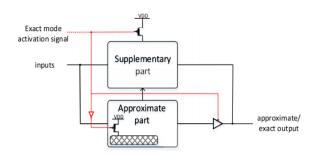
Fig .3. Block diagram of the proposed approximate 4:2 compressors
